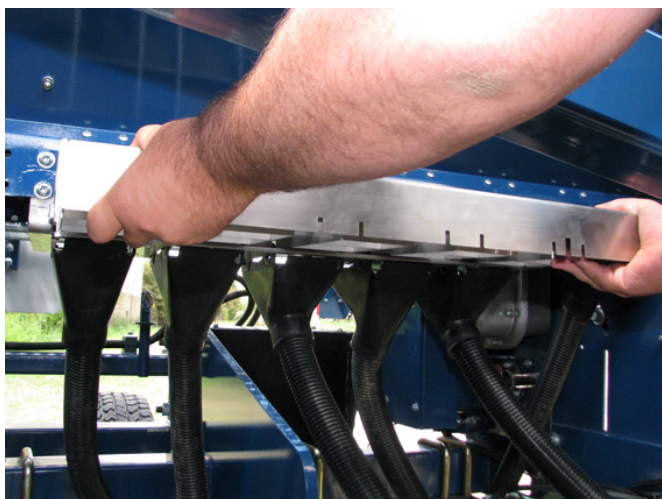
Agrowplow Area manager Colin Hercott shows off the new generation Agrowdrill’s calibration trays. The new tray system makes calibration on the new drill faster and easier.
